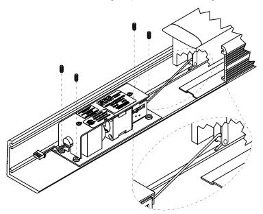
ELECTRICAL DATA 24VDC +/- 10% 1.5A Inrush / 200mA holding RED (+) BLK (-) PATENT #8,851,530
