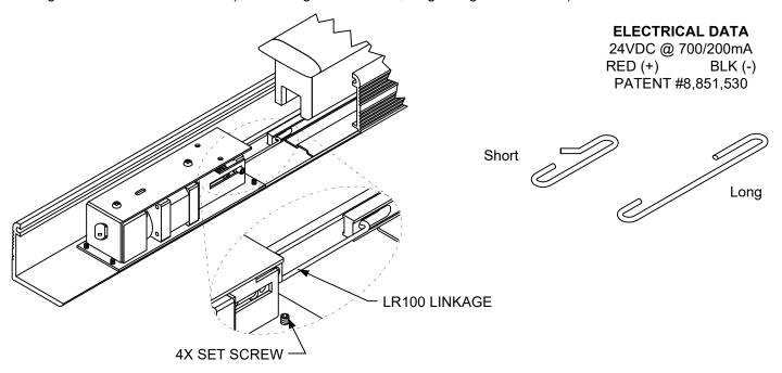
Carefully slide the assembly back out until the linkage <u>JUST</u> makes contact with the latch retraction rod. Tighten set screws.
