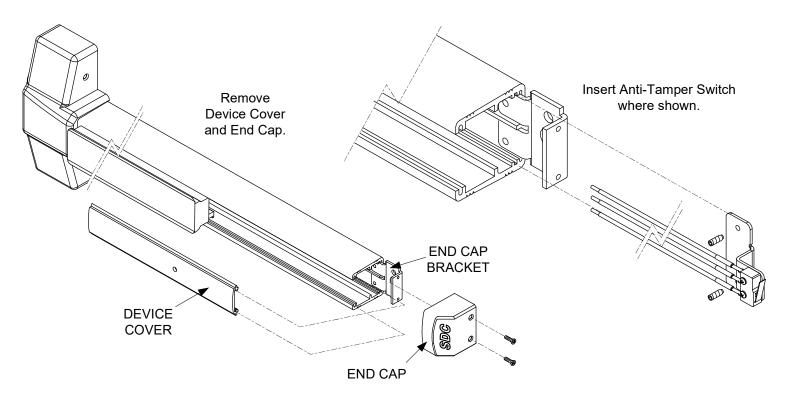
Insert the S6000-ATS assembly into the device as illustrated above. Slide the End Cap over the End Cap Bracket. Position the S6000-ATS assembly so that the switch arm makes contact with the inside surface of the End Cap. While the assembly is in position fasten the provided set screws on the S6000-ATS to lock it in place.
