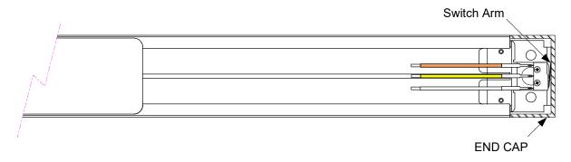
Once the S6000-ATS monitoring switch assembly is properly secure within the device, wire the switch and re-install the Device Cover and End Cap.
