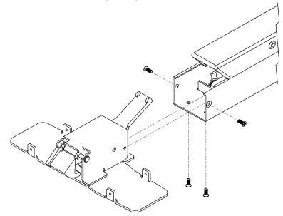
Remove the front two screws connecting the push pad to the housing. Route the wires along the side of the housing and out the back. Slide the LRTS2R into the housing <u>under</u> the push pad mounting bracket.
