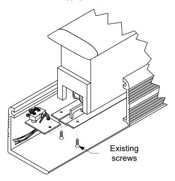
Replace existing screws with the mounting screws supplied with the switch kit and install the kit in the existing holes where shown.
