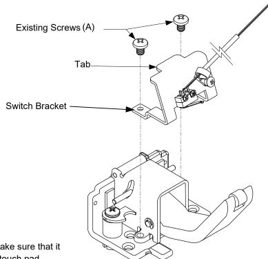
Route wires cable along the side of the device. Make sure that it doesn't interfere with the normal operation of the touch pad.
