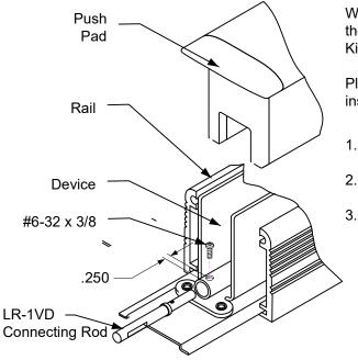
When retrofitting to existing vertical rod devices, adjustment of the rods are required for proper assembly of the LR100VDK Kit.
