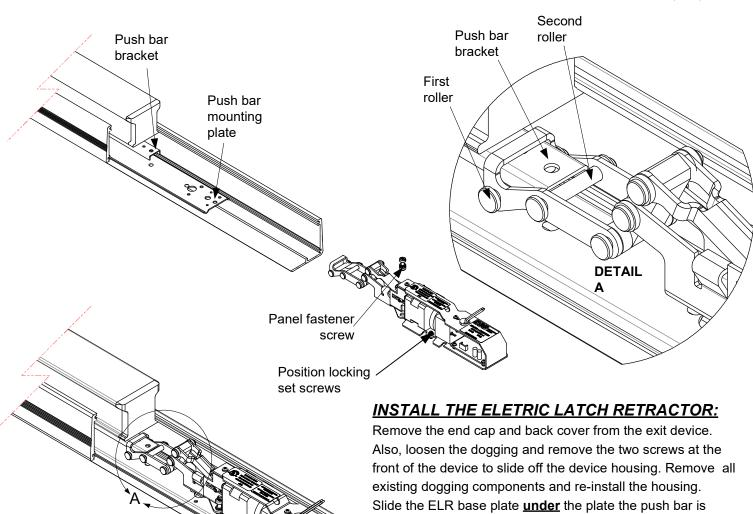
mounted to and attach the supplied panel fastener screw to the existing hole where the dogging was mounted.
