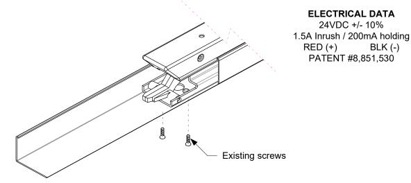
Slide the ELR assembly into the housing and under the hinge bracket. Position the roller at the front of the ELR under the pivot arm of the push bar.
