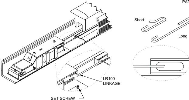
Back the assembly out until the linkage <u>JUST</u> makes contact with the latch retraction rod. Tighten set screws. Replace cover plate and end cap.
