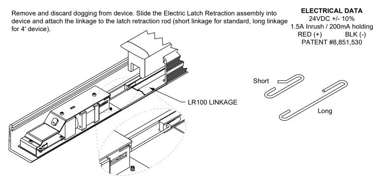
Slide back the assembly out until the linkage <u>JUST</u> makes contact with the latch retraction rod. Tighten set screws.
