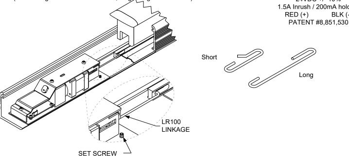
Slide the assembly back until the linkage <u>JUST</u> makes contact with the latch retraction rod. Tighten set screws. Replace cover plate and end cap.
