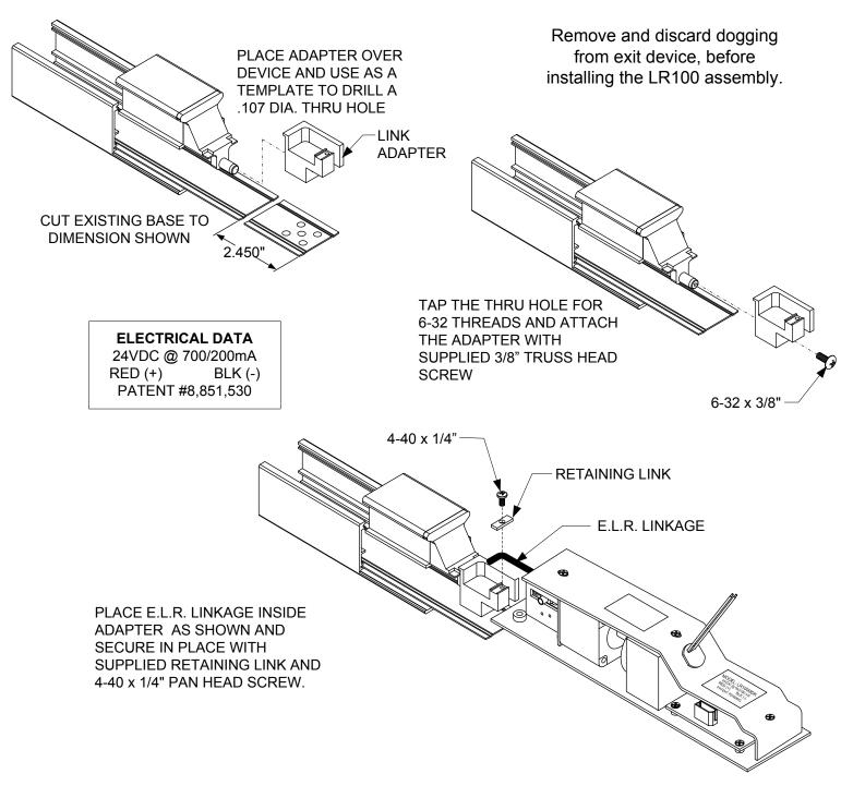
AFTER ATTACHING LINKAGE, POWER THE UNIT. THIS WILL CAUSE THE E.L.R. TO PULL INTO THE EXIT DEVICE. DEPRESS THE PUSH PAD TO PROPERLY POSITION THE E.L.R. MANUALLY PULL THE E.LR. ASSEMBLY BACK TIGHTEN THE SET SCREWS TO LOCK THE E.L.R. IN PLACE. TEST FUNCTION OF E.L.R. BY APPLYING POWER TO VERIFY THAT THE E.LR. ASSEMBLY RETRACTS THE PUSH PAD AND LATCH
