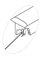
Back the assembly out until the linkage <u>JUST</u> makes contact with the latch retraction rod. Tighten set screws.
