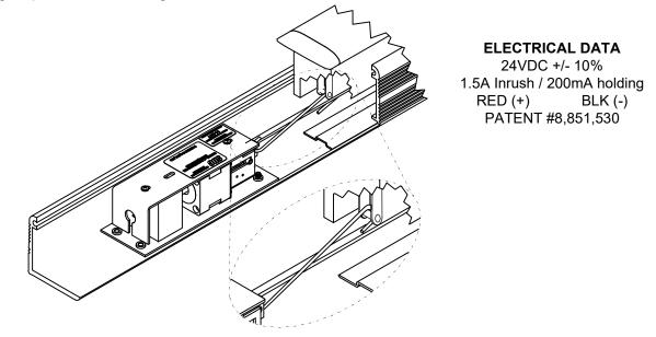
Carefully slide the assembly back out until the linkage <u>JUST</u> makes contact with the latch retraction rod. Tighten set screws.
