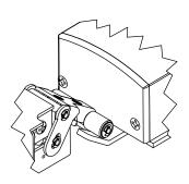
Slide the ELR unit outwards till the rollers just make contact with the forked activation tab. Slide the fixation plate against the ELR unit and tighten the set screws.
