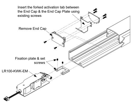
Depress the touchpad completely and slide the ELR unit in over the forked activation tab.
