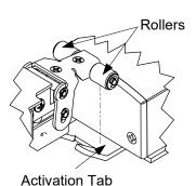
Energize the ELR unit which will bring the rollers down towards the activation tab.
