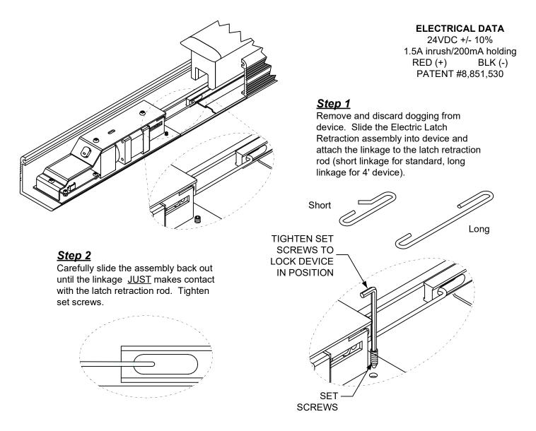
**<u>Retrofit Installation Note:</u>** 42" or 48" exit devices that have been modified to fit a 36" or smaller opening, may not have the required space to fit the standard E. L. R. assembly. Always verify the distance from the end of the touchpad to the end rail, and if necessary, consult with the factory for appropriate selection.
