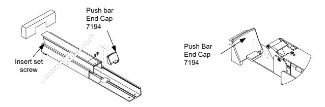
Install the ELR roller clevis assembly over the top of the push bar end cap 7194. When properly aligned, tighten the two supplied set screws to lock in place as shown in detail A. Wire the unit and test operation. Reinstall the new cover and end caps. Orient the cover and end caps as shown.
