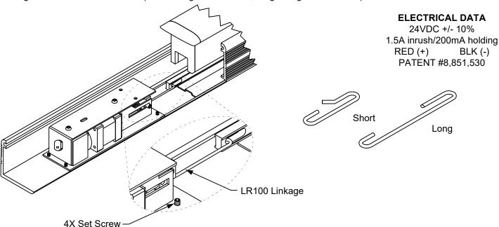
Carefully slide the assembly back out until the linkage <u>JUST</u> makes contact with the latch retraction rod. Tighten set screws.
