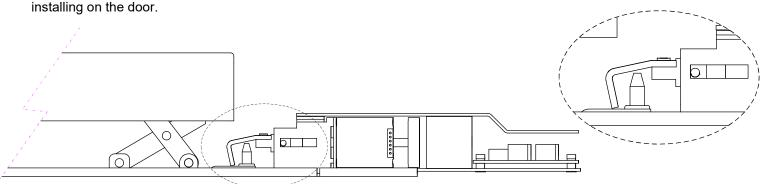
When retrofitting to existing vertical rod devices, adjustment of the rods are required for proper assembly of the LR100FRK Kit. Please see the SDC website (www.sdcsecurity.com) for installation tips and photographs of installing.
