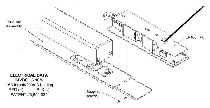
Make sure the linkage at the end of the ELR unit engages the shaft on the Exit Device as shown. Carefully slide the Push Bar Assembly with attached ELR unit back into the extrusion and re-attach the head. Test the unit before re-
