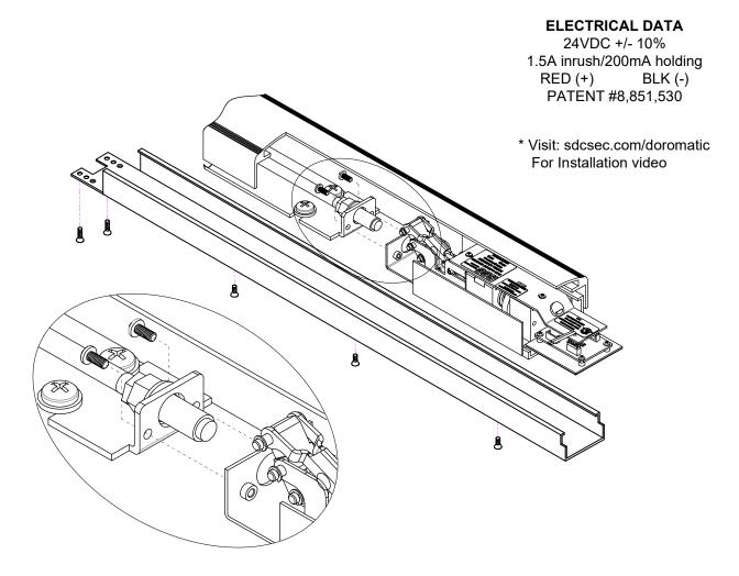
When retrofitting to existing vertical rod devices, adjustment of the rods is required for proper operation of the Electric Latch Retractor. Once the unit is properly installed, energize it so the latch is dogged down, then reconnect the vertical rods to the device and make the proper adjustments.
