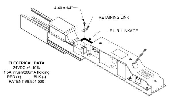
Once the linkage is attached, power the unit. This will cause for the E.L.R. to pull towards the exit device. Depress on the push pad, by doing so will properly position the E.L.R. into the appropriate working position. Pull back on the E.L.R. assembly to remove any slack. Then fasten the set screws on the assembly to secure the kit into the device. Release push pad and verify operation by de-energizing and re-energizing the E.L.R. kit to verify that the kit is properly retracting the latch.
