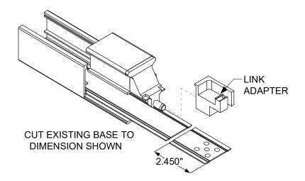
Remove and discard dogging from exit device, before installing the LR100 assembly. Tap a Thru Hole to accept a 6-32 thread and attach the adapter using the supplied 6-32 x 3/8" Truss Head Machine Screw.
