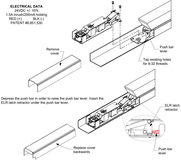
When retrofitting to existing vertical rod devices, adjustment of the rods is required for proper operation of the Electric Latch Retractor. Once the unit is properly installed, energize it so the latch is dogged down, then reconnect the vertical rods to the device and make the proper adjustments.
