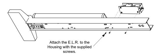
**Note for Vertical Rod Devices:** Once the ELR is properly installed, disconnect the vertical rods from exit device and energize the ELR so that the push pad is dogged down. This will allow for proper alignment of the vertical rods. Reconnect the vertical rods to the device and make the proper adjustments.
