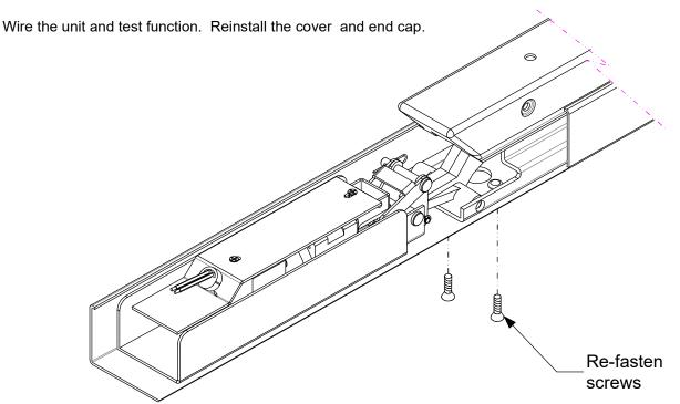
When retrofitting to existing vertical rod devices, adjustment of the rods is required for proper operation of the Electric Latch Retractor. Once the unit is properly installed, energize it so the latch is dogged down, then reconnect the vertical rods to the device and make the proper adjustments to the rods.
