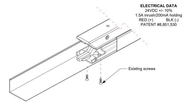
Slide the ELR assembly into the housing and under the hinge bracket. Position the roller at the front of the ELR under the pivot arm of the push bar.
