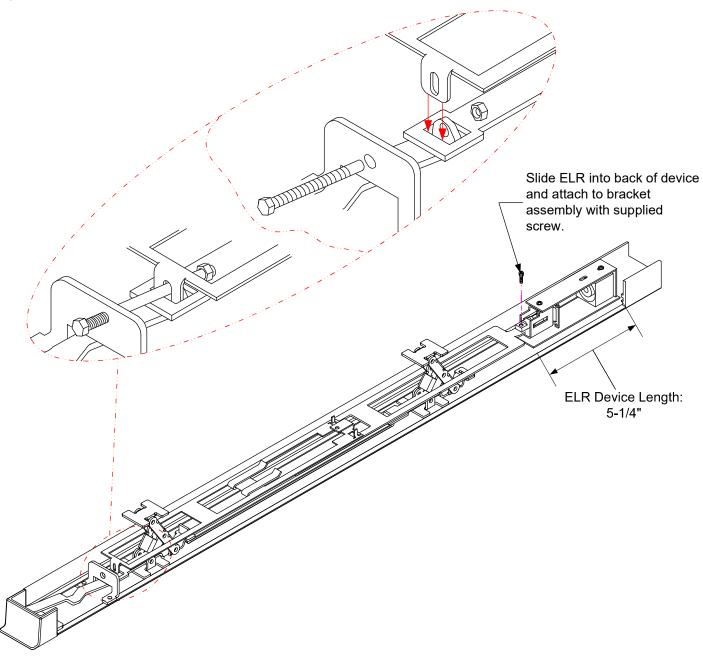
Apply power to the ELR unit to make it draw the sliding latch bracket back to the open position. Secure in position by tightening the set screws in the ELR assembly.
