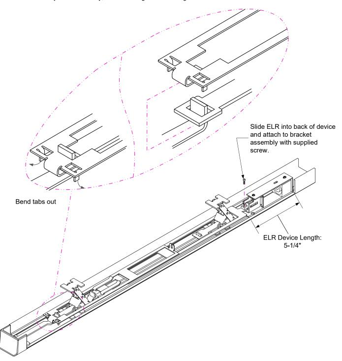
Apply power to the ELR unit to make it draw the sliding latch bracket back to the open position. Secure in position by tightening the set screws in the ELR assembly.
