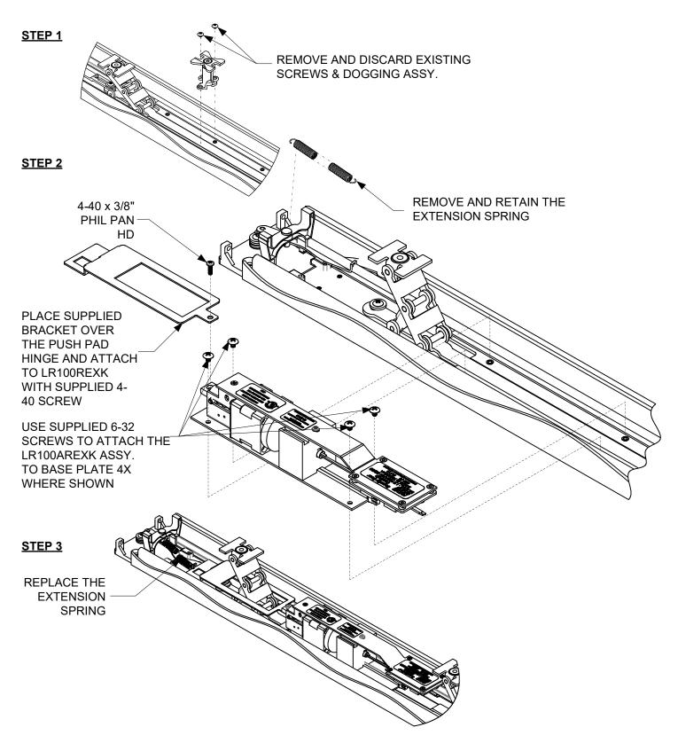
When retrofitting to existing vertical rod devices, adjustment of the rods is required for proper operation of the Electric Latch Retractor. Once the unit is properly installed, energize it so the latch is dogged down, then reconnect the vertical rods to the device and make the proper adjustments to the rods.
