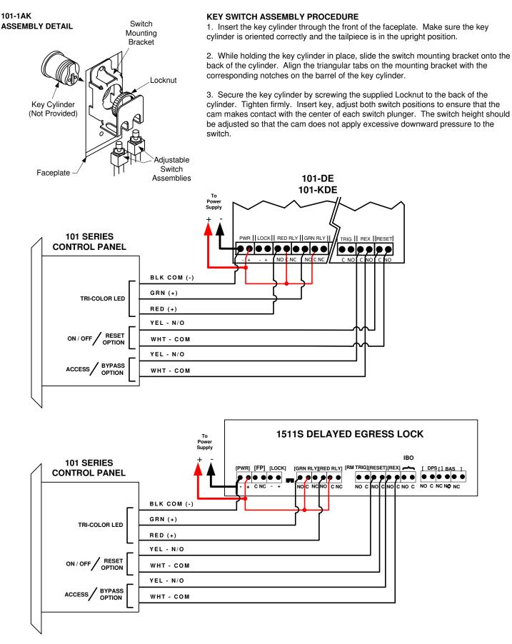
NOTE: AUDIBLE SHUNT OPTION IS NOT WIRED TO DE LOCK.
