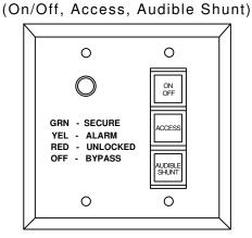
20 GAUGE STAINLESS STEEL SPDT, 2A @ 30VDC SPDT, 5A @ 30VDC -AUDIBLE SHUNT LAMP: 40mA @ 28VDC 93dB @ 1 METER, 20mA @ 28VDC TRI-COLOR LED, 30mA @ 12/24VDC -GREEN (SECURE) -AMBER (ALARM/DOOR LOCKED) -RED (ALARM/DOOR UNLOCKED)
